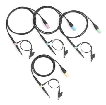
The THP0301 probes are 300 MHz, 10X passive voltage probes with 10 M $\Omega$  input resistance. These probes are for use with the THS3000 Series oscilloscopes and are color coded to match the oscilloscope's channel input connectors, front-panel channel selector buttons, and the displayed waveforms.
